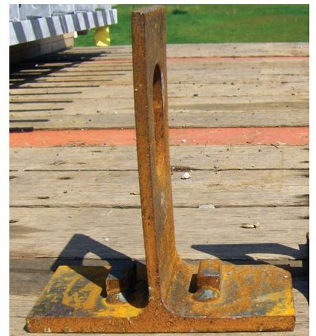
Lifting device made from WT shape.
