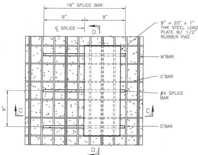
Plan view of load plate set-up on spliced panel
