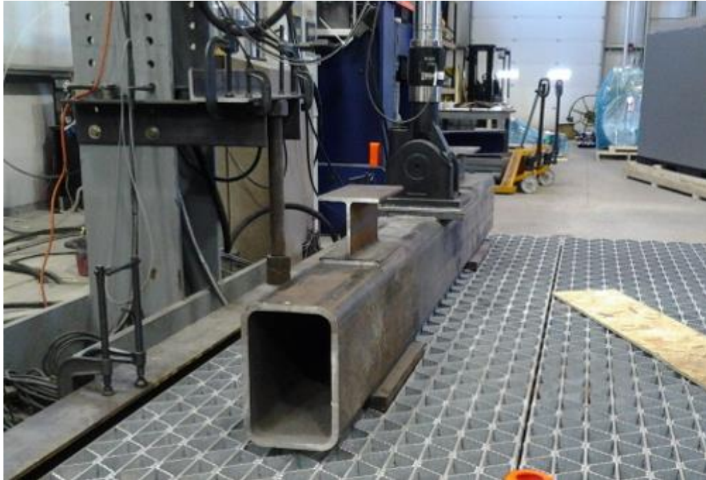
Figure 4.8 - Laboratory set-up for Test #1 with load at mid span of panel 37R5-A1
